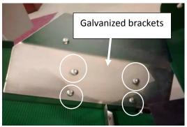
20. With the galvanized bracket now bolted to the conveyor, lift it in place so that it can be attached to the processor. A scissor jack or car jack can be used to aid in lifting the conveyor up into place so the mounting holes align.
