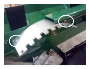
16. Install the 2/4 way splitter bottom support as shown below. The handle can also be installed at this point along with the 2/4 way splitter itself.
