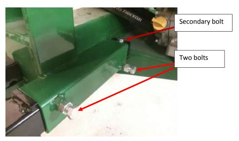
30. Attach tongue jack as pictured below. There are two bolts that hold it securely to the tongue. The leg stand can be used when the processor is in operation.
