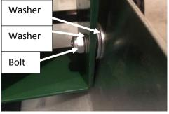
21. The top half of the conveyor can now be installed to the bottom half by bolting it at the seam using the hardware shown below. Be sure to install one of the washers in between the top and bottom conveyor. The nut should be left loose so that the bolts act as a hinge and allow the conveyor system to fold in half. Also, be sure that the conveyor is looped around the top roller.
