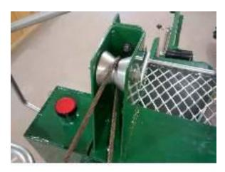
28. Attach the hook to the hook attachment point on the conveyor.
