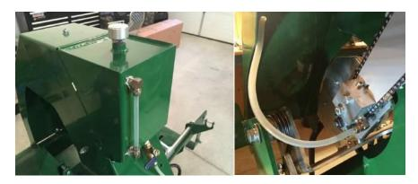
9. Install the back plate, reinforcement bracket, and the top pulley housing to the chainsaw bar guard using the bolts provided. Tighten all bolts including the bolts from step 7.
