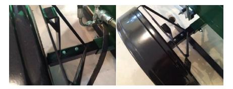
5. The four lug nuts of each wheel should be torque to 90 ft-lbs.
