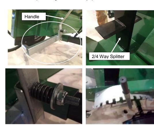
17. Install log deck roller assembly as shown in below images.
