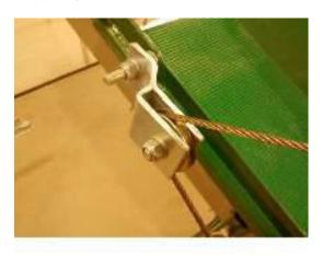
27. Remove the large pulley from the pulley housing on top of the chain guard, feed the cable through and re-install the pulley.
