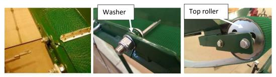
22. The top half can now be latched to the bottom half as shown below. Once latched in place, one person can begin to lift the conveyor up so another person can slide the support leg in place and latch the chain.
