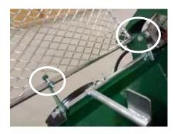
15. Install the notched plate on the processor with the 2 nuts and bolts provided. This plate is used to lock the handle in place which holds the 2/4 way splitter is at the desired height.
